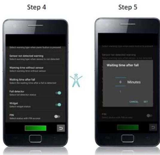
Change the time between a fall is detected and the alarm starts. For testing, we recommend to change the default value to 0 sec, this way the alarm bell sounds immediately.
