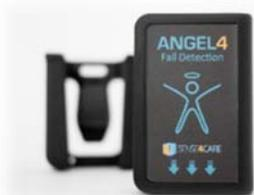
The Device has not button nor other manual control to interact with. All actions should be done through the smartphone application, to turn it on and turn it off.
